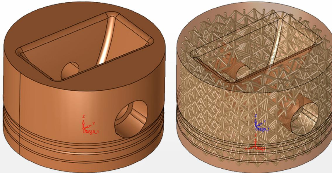
3D metal additive delivers 35% lighter-weight through internal latticework and partially sintered metal materials.
