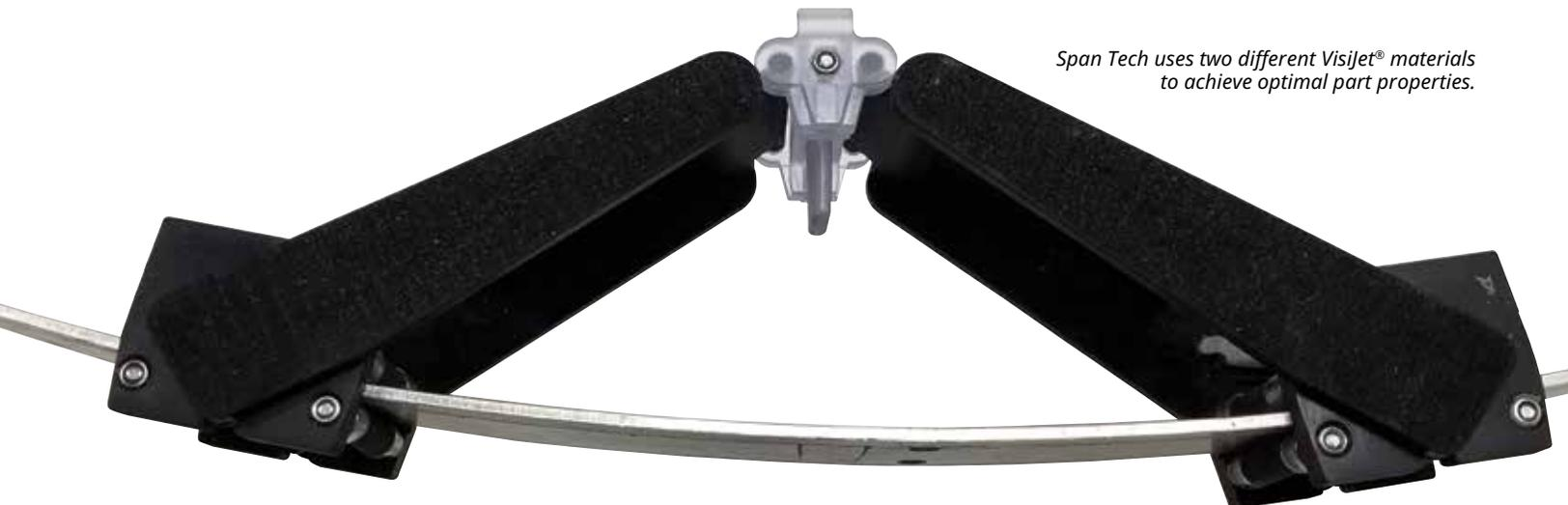
*Span Tech 3D prints its conveyor prototypes in full size using the ProJet® MJP 2500 Plus.*
