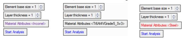
A **Purple** color means that the system did not find any calibration data for this material, and therefore it uses the next best calibration data from the list of calibrated materials. For example, if the material is recognized as any type of titanium, then it will use the generic titanium calibration.
