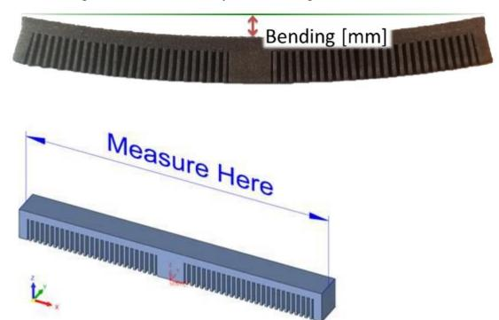
Avoid measuring near the corners of the part, as corners are further deflected.
