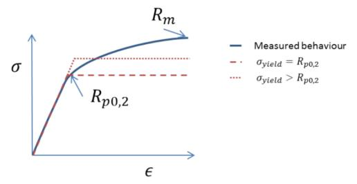
The model of Ideal Plasticity assumes that in most cases, the stress value where a plastic deformation of 0.2% (Rp0.2) will occur, is identified as the yield (yield stress is the stress at which a material begins to have a plastic deformation). From then on, the stress is constant.
