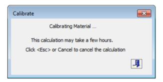
Wait for this to finish. At the end, the text Calibrated will be displayed at the bottom of the dialog.
