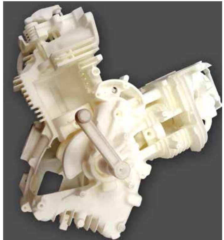
The addition of SLS has transformed Briggs & Stratton's prototyping capabilities, unlocking unprecedented productivity in product development. Pictured left is a static engine cover. Pictured right is a 3/4 scale V-twin engine that turns with the crank handle and was printed as an assembly; only the pushrods were printed separate.
