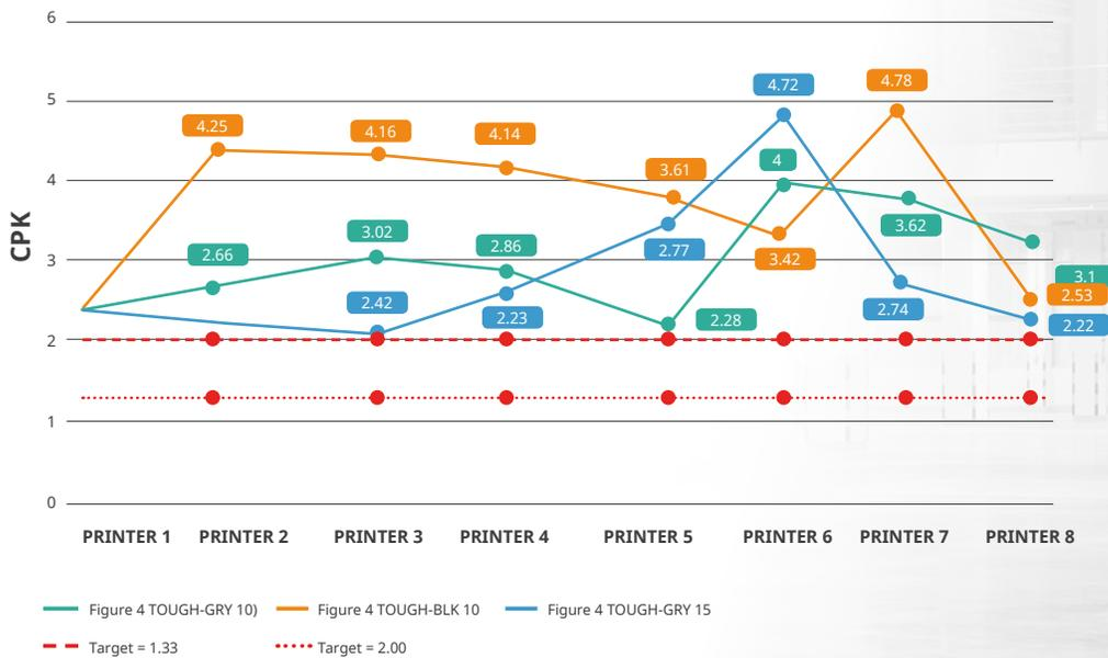
Results from three Figure 4 printers with three different materials consistently deliver a Cpk > 2. This equals 0.002 parts per million are out of spec (Preliminary data).
