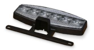
Using the SLA 3D printer and VisiJet® SL Clear material the company has shifted its lens prototyping from direct machining in plastics to 3D printing to deliver superior prototypes, faster. With a lacquer clear coat on the printed lenses, TecNiq was able to match the surface quality of its manufactured products.
