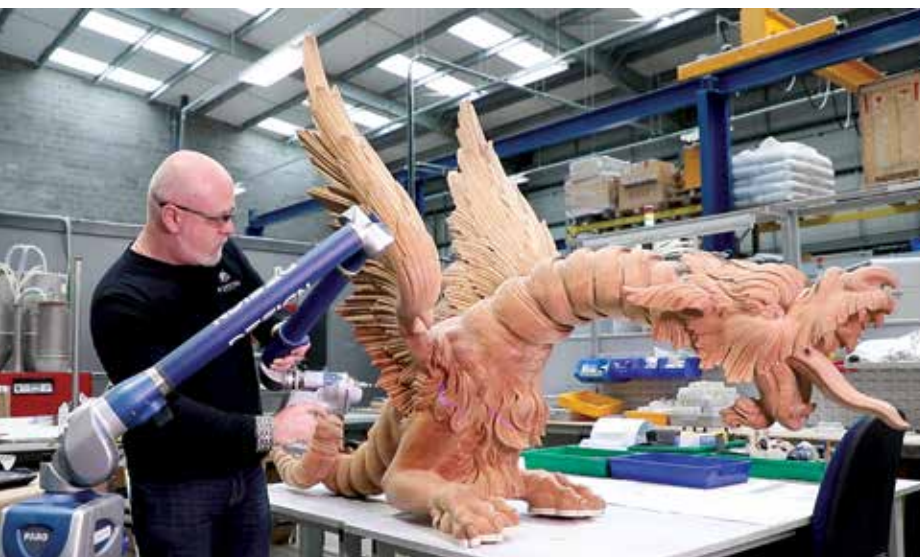
The carved wooden dragon was 3D scanned as part of a reverse engineering workflow.
