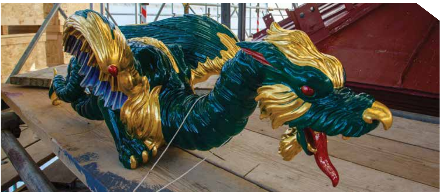
After 3D printing, the dragons were finished and hand painted by 3D Systems' High Wycombe finishing department.
