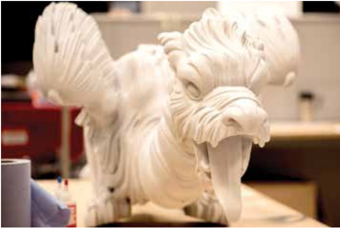
SLS 3D printing solved the quality, weight, time and cost concerns of the HRP restoration team.
