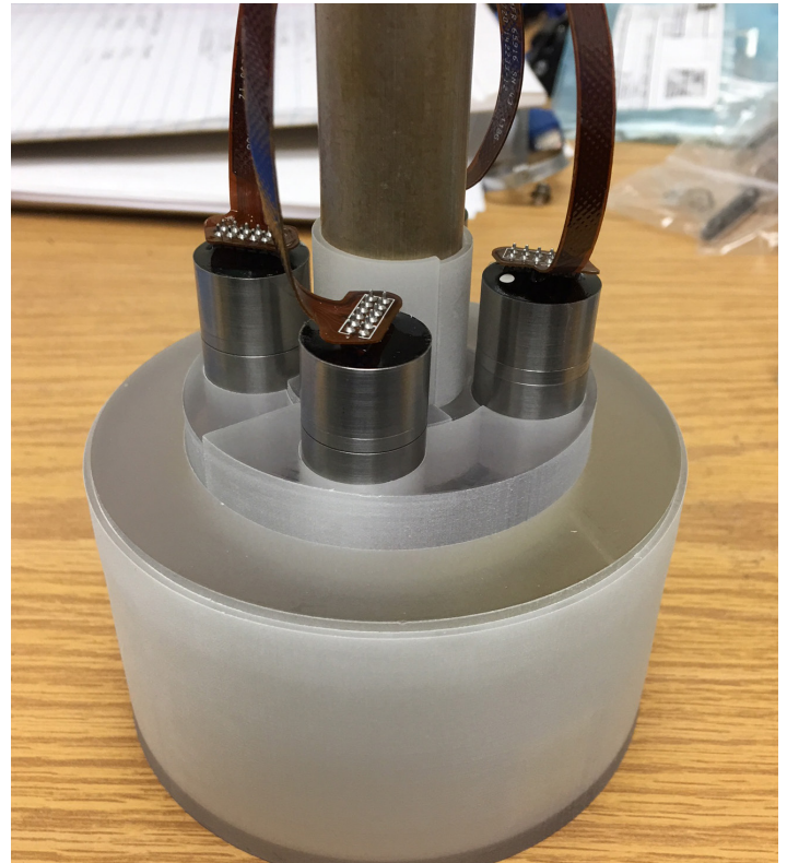
A sealable, watertight 3D printed cover ensures costly motors are not damaged during shipping or cleaning.
