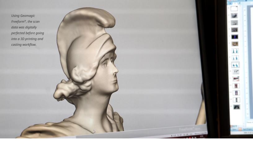
"Whenever we did something that didn't come out quite right, we pressed Control-Z to undo the move and redid it until we got it right," Carter said. The team designed the mounting hardware in SOLIDWORKS CAD system and exported STEP files which were imported into Freeform and subtracted from the Britannia model. Freeform was then used to reduce the model to half its original size.
