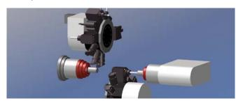
**Dual Turrets, Dual Spindles:** These machines are typically configured with upper and lower turrets, which enable pinch turning, so roughing operations can be done in half the time. The machine will have up to 8 axes: X, Y and Z on the upper turret, X and Z on the lower, a third Z (or A or W) on the subspindle for part transfer, and C rotary on each spindle.
