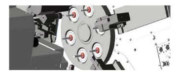
The goal with these is to eliminate tool changes, and minimize X and Y motion. Each spindle has its own bar feeder, which pushes material out through a collet or guide bushing. Limited operations are done at each tool station, then the barrel rotates so the part moves to the next tool group – indexing to the next position – until the part is finished, cut off, and dropped at the 6th station
