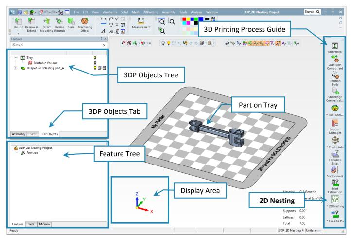
3. From the **3DP Objects Tree** hide the Printable Volume (*pick* the yellow bulb to hide). This hide the red wireframe which represents the printing volume.
