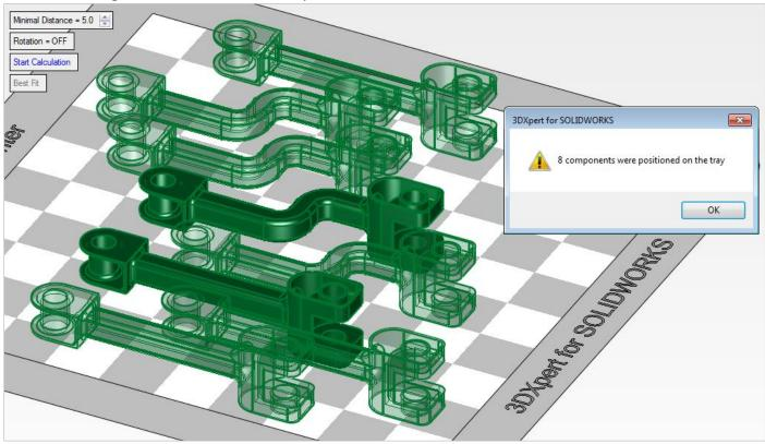
In case that not all the parts can be nested on the tray, a relevant message will appear and the rest of the part remain out of tray (these parts can be removed):
