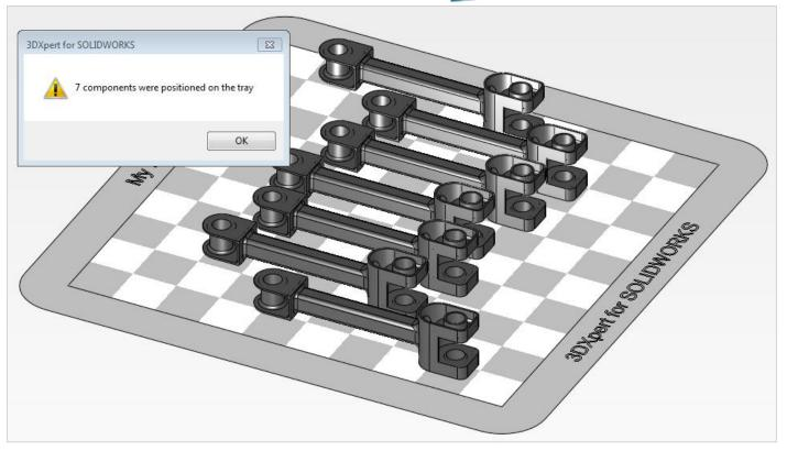
Note the message, specifying that 7 components were positioned on tray in this orientation, *Pick* OK.
