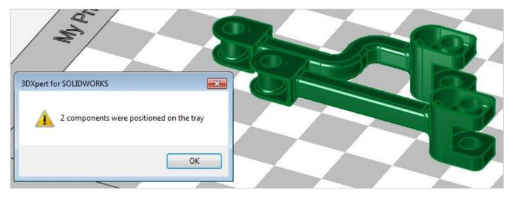
Note that in this case (of more than one part), 2D Nesting is only arranging the parts on tray, Pick OK.
