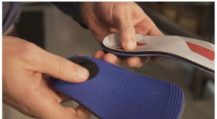
"The build volume, material options and precision of the printer are critical factors for us," says Salmon. "Having a large build volume allows us to maximize the number of insoles per print. The more we can pack into a 24-hour print cycle, the more cost effective it becomes. The massive amounts of SLS materials allow us to find the right option for each application, while having the ability to be agile and switch materials within a few hours."
