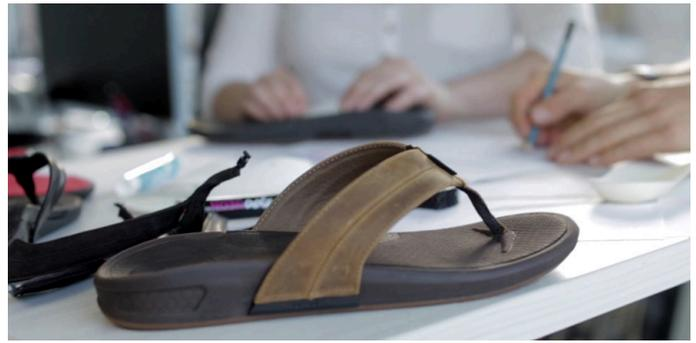
arch supports with the other elements produced using more traditional means. The straps and toe thongs are produced with traditional injection-molded techniques, but are still customizable. The straps can be adjusted and replaced, and the toe thongs are assigned to one of three positions based on the customer's smart phone photos.
