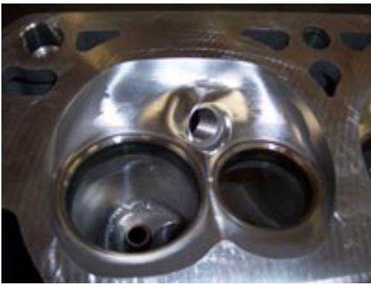
Completed combustion bowl
