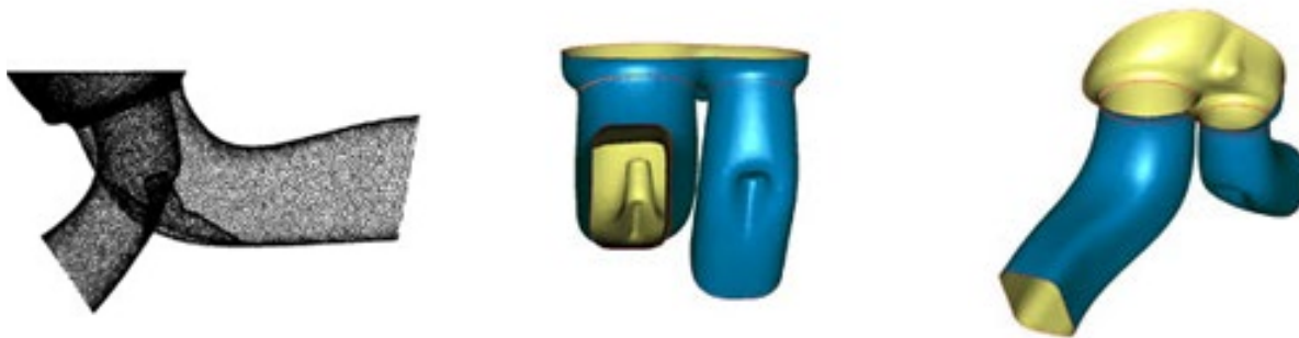
From left to right: Internal detail of cylinder head port in Geomagic Studio; side view of cylinder head port as a 3D point cloud; intake, exhaust and combustion bowl assembly digitally reconstructed in Geomagic Studio
