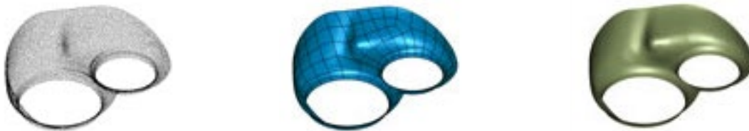
Point cloud, mesh and surface of combustion bowl in Geomagic Studio
