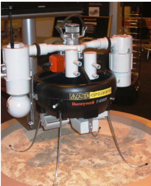
The white parts on this finished version are 3D printed as production parts using SLS, including the air-foil vanes that were printed as complete assemblies
