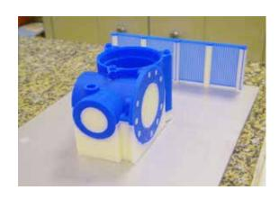
Image above: One 3D printed wax part with white was supports
